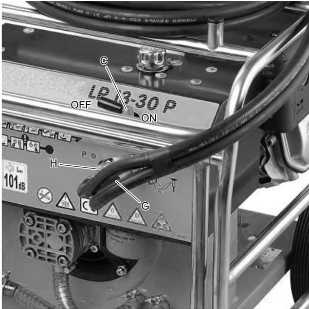
The by-pass valve (C) must be in the OFF position when starting and in the ON position when using the machine.
