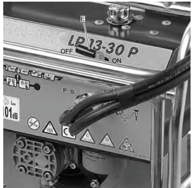
5. Pull out the starter rope (D) until it resists. Release the handle so the starter rope goes back again, and then pull the starter rope until the engine starts.
