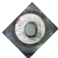
Arbor Hole Out-Of-Round Blade not properly tightened or seated on arbor.
