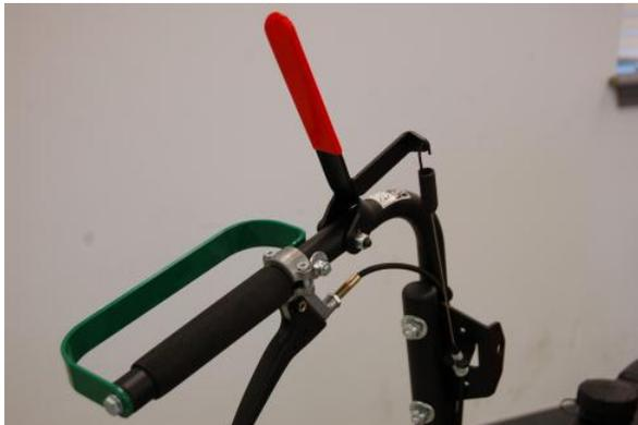
Blade Clutch Lever located on left handlebar
