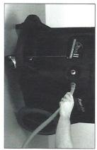
CAUTION: Check hose connection regularly to make sure it is tinue to flow until the suction is decreased. sure. If the hose should come loose, water in the hose will consecurely fastened. The pump discharges water at high pres-
