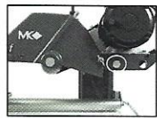
(D) For maximum cutting length, the Cutting Head should be in the front pivot hole and the Post should be in the rear post retaining hole.
