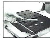
(A) Loosen Adjustable Cutting Guide retaining thumbscrew and place it over the Movable Cutting Table Ruler/Stop
