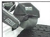
(B) Set cutting depth approximately 1/4 to 1/2 inch below the surface of the Movable Cutting Table
