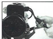
(B) Connect the Water Pump power cord to the connection found on the back of the motor
