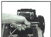
(A) Connect the Cooling Transfer Tube to the inlet connection of the Blade Guard
