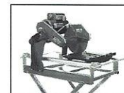
(B) Remove Water Basin and place saw on stand
